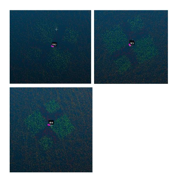
$\label{eq:note} \underline{\text{NOTE}}$  Colorization effected the point cloud resolution.
