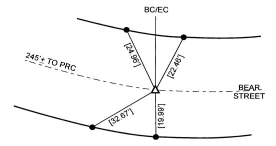
▲ = SET GEAR SPIKE & WASHER W/ TAG STAMPED LS 5411 PER R1 AFTER CONSTRUCTION
