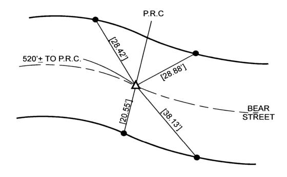
▲ = SET GEAR SPIKE & WASHER W/ TAG STAMPED LS 5411 PER R1
