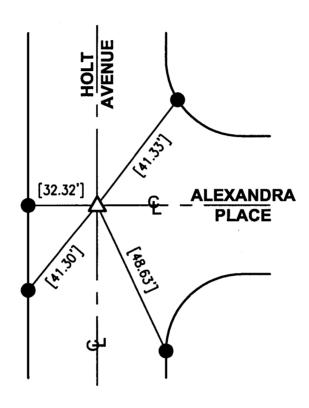
↑ FD NOTHING, SET GEAR SPK & W, STAMPED "LS 5411" PER TIES ON R-1, FLUSH, AFTER CONSTRUCTION.
