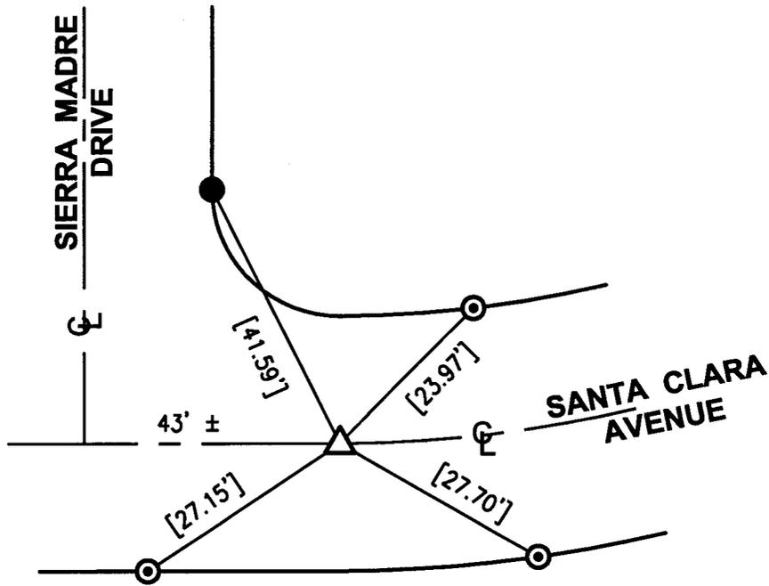
△ FD NOTHING, SET GEAR SPK & W, STAMPED "LS 5411" PER TIES ON R-1, FLUSH, AFTER CONSTRUCTION.
