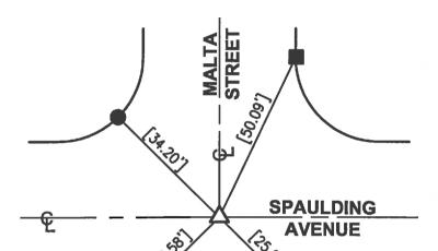
$\Delta$  set gear spike & washer "LS 5411" per ties on R-1, flush, after construction.
