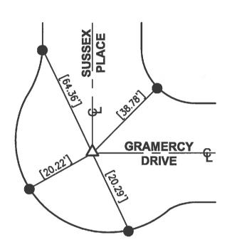
△ SET GEAR SPIKE & WASHER "LS 5411" PER TIES ON R-1, FLUSH, AFTER CONSTRUCTION.
