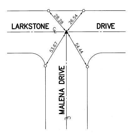
NOTE: THESE TIES ARE FOR THE PURPOSES OF PERPETUATING THE FOUND MONUMENTATION. NO CLAIM IS MADE TO THE RELATIONSHIP OF THE POINTS OR LINES SHOWN HEREON TO THE TRUE BOUNDARY LOCATIONS.
