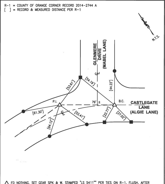
↑ FD NOTHING, SET GEAR SPK & W, STAMPED "LS 5411"" PER TIES ON R-1, FLUSH, AFTER CONSTRUCTION.
