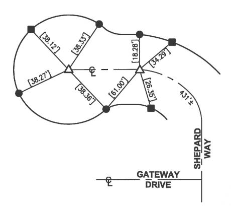
△ SET GEAR SPIKE & WASHER "LS 5411" PER TIES ON R-1, FLUSH, AFTER CONSTRUCTION.
