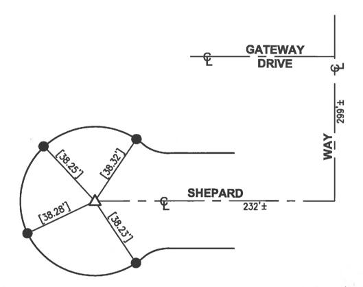
△ SET GEAR SPIKE & WASHER "LS 5411" PER TIES ON R-1, FLUSH, AFTER CONSTRUCTION.
