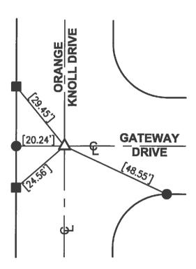
△ SET GEAR SPIKE & WASHER "LS 5411" PER TIES ON R-1, FLUSH, AFTER CONSTRUCTION.
