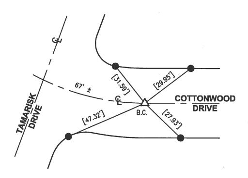
↑ FD NOTHING, SET GEAR SPK & W, STAMPED "LS 5411"" PER TIES ON R-1, FLUSH, AFTER CONSTRUCTION.
