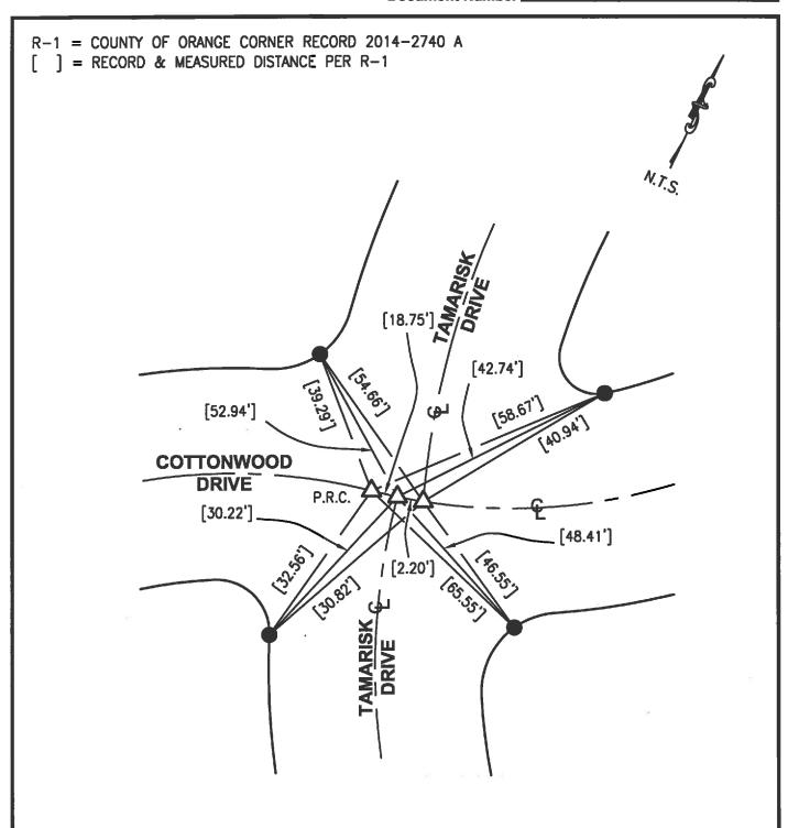
A FD NOTHING, SET GEAR SPK & W, STAMPED "LS 5411"" PER TIES ON R-1, FLUSH, AFTER CONSTRUCTION.
