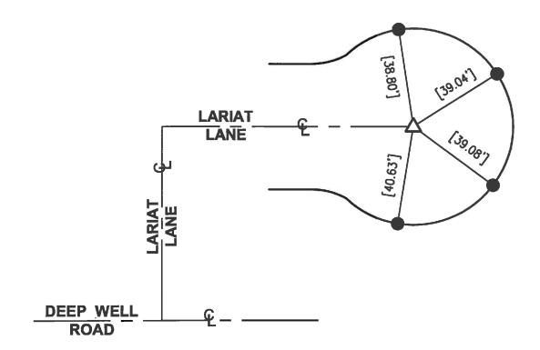
↑ FD NOTHING, SET GEAR SPK & W, STAMPED "LS 5411"" PER TIES ON R-1, FLUSH, AFTER CONSTRUCTION.
