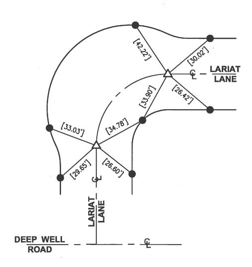
↑ FD NOTHING, SET GEAR SPK & W, STAMPED "LS 5411"" PER TIES ON R-1, FLUSH, AFTER CONSTRUCTION.
