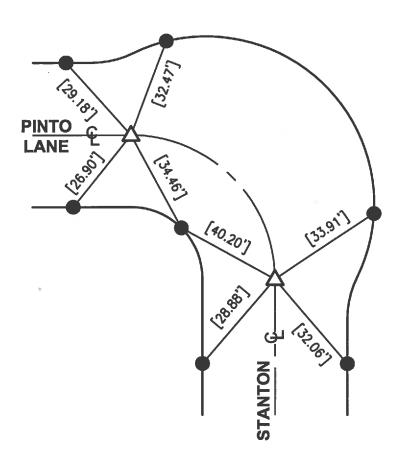
△ FD NOTHING, SET GEAR SPK & W, STAMPED "LS 5411"" PER TIES ON R-1, FLUSH, AFTER CONSTRUCTION.
