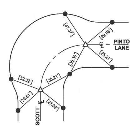
↑ FD NOTHING, SET GEAR SPK & W, STAMPED "LS 5411"" PER TIES ON R-1, FLUSH, AFTER CONSTRUCTION.
