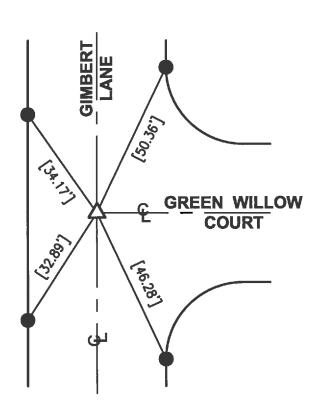
△ FD NOTHING, SET GEAR SPK & W. STAMPED "LS 5411"" PER TIES ON R-T, FLUSH, AFTER CONSTRUCTION.
