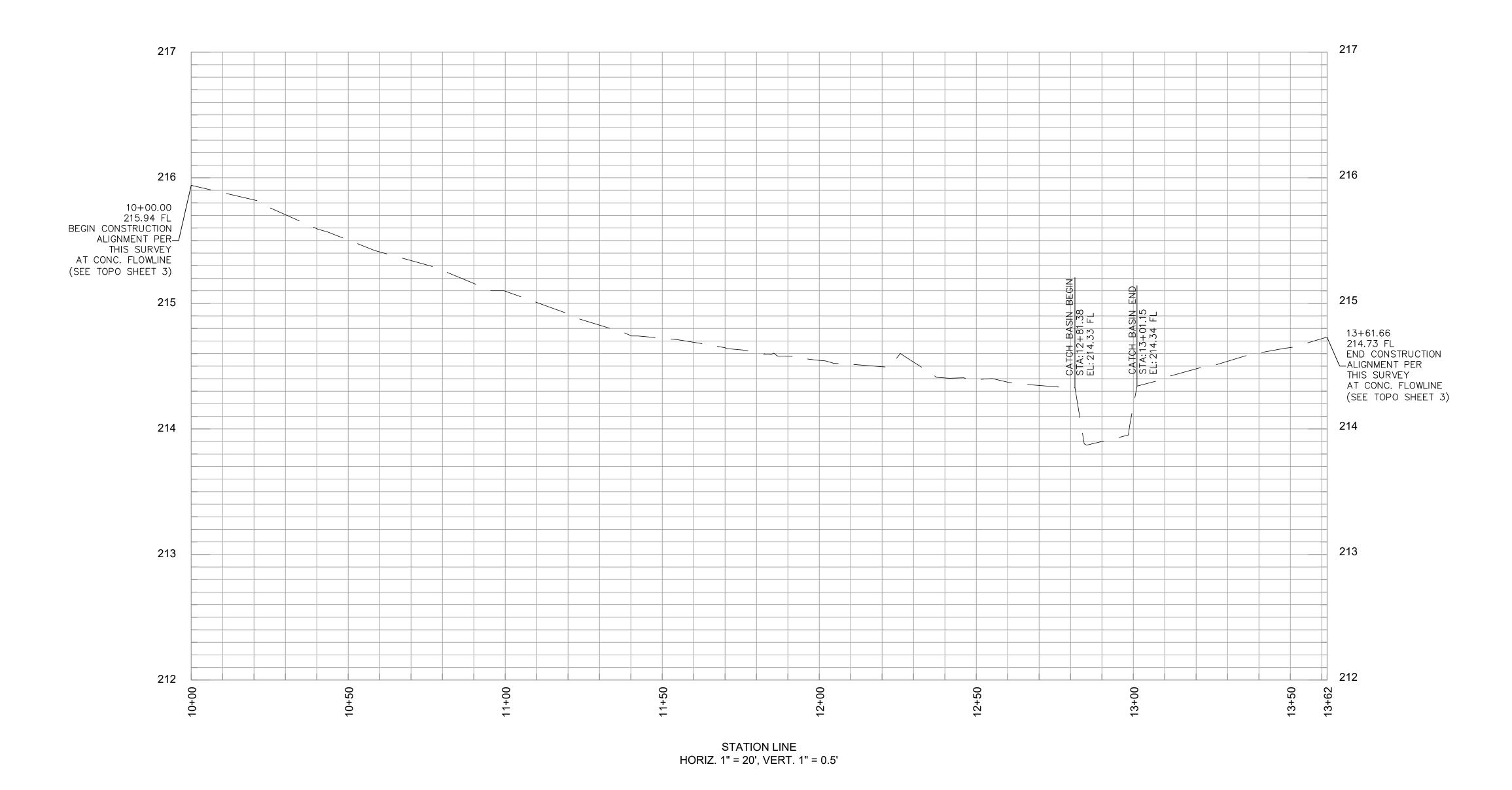
NOTE: THE ALIGNMENT FOR THIS PROFILE WAS DEVELOPED HOLDING A STATION OF 10+00 AT THE NW'LY END OF THE EXISTING CONCRETE FLOWLINE OF THE W'LY SIDE OF FLINT DR. AND INCREASING S'LY AND E'LY AS SHOWN ON SHEET 3
