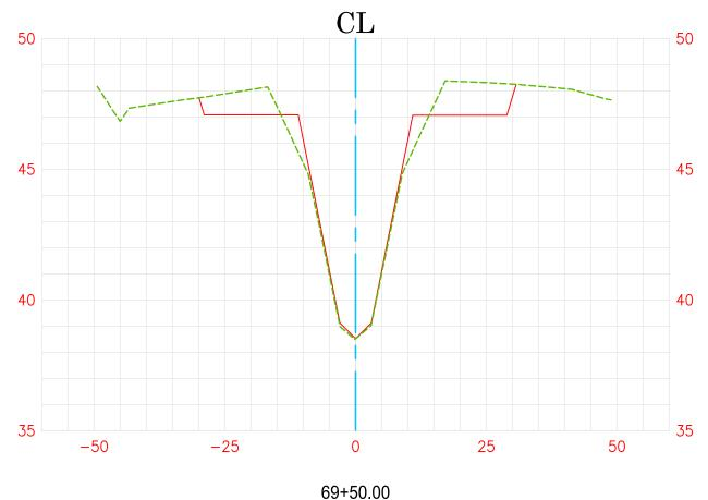
2019 Channel Survey As-Built Plan
