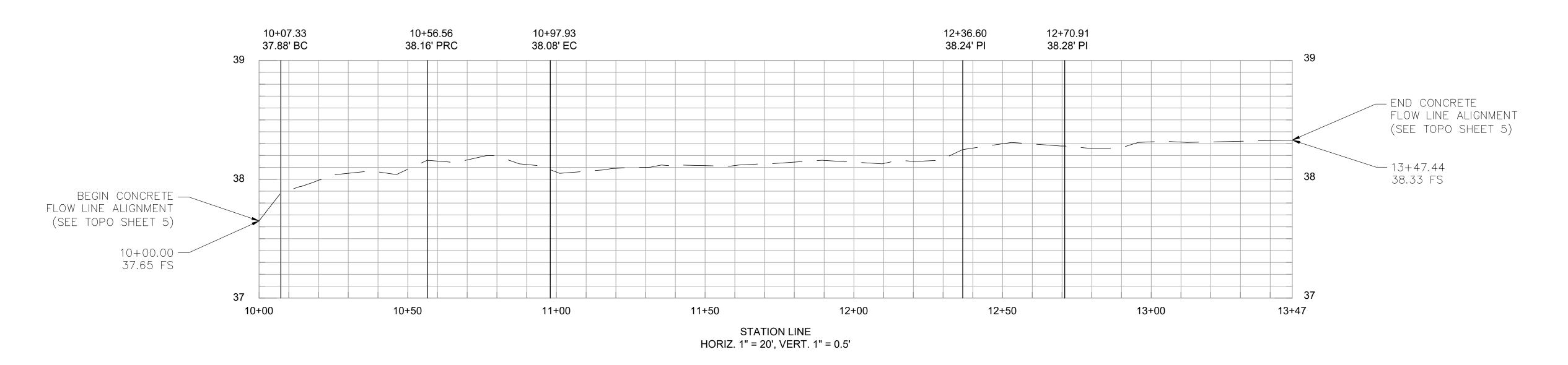
NOTE: THE ALIGNMENT FOR THIS PROFILE WAS DEVELOPED HOLDING A STATION OF 10+00 AT THE W'LY END OF THE EXISTING CONCRETE FLOWLINE OF THE N'LY SIDE OF BOLSA AVENUE FRONTAGE ROAD AND INCREASING E'LY AS SHOWN ON SHEET 5
