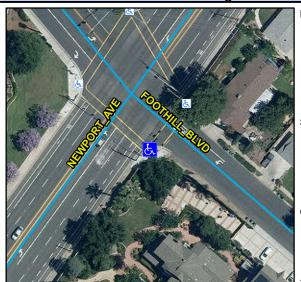
Possible Solutions: Remove & Replace Curb Ramp With Two New Directional Ramps or Equivalent. Remove & Replace Gutter.
