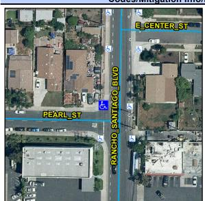
Possible Solutions: Remove & Replace Curb Ramp With Two New **Directional Ramps or Equivalent.**
