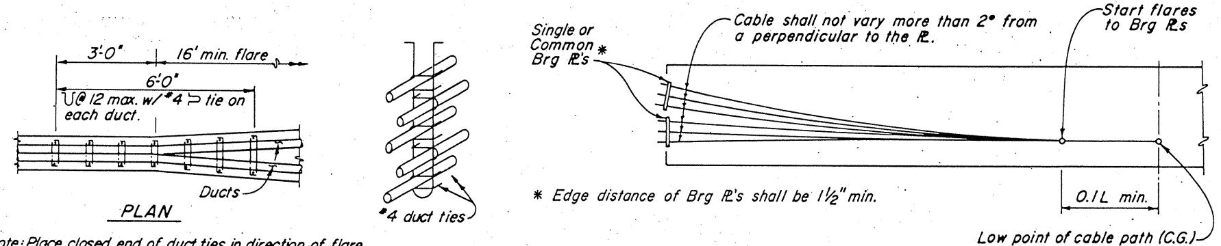
Note: Place closed end of duct ties in direction of flare
