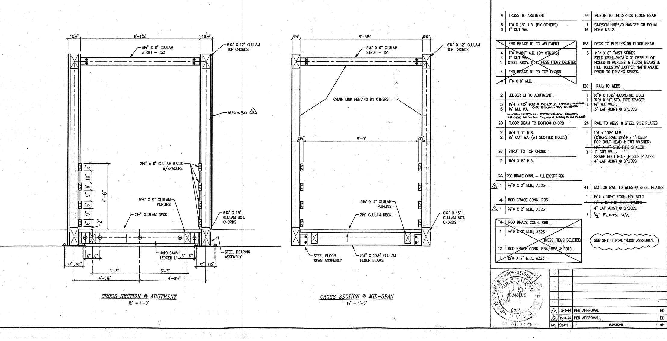
DESIGN CRITERIA LIVE LOAD : 85 PSF. GLULAM SPECIFICATIONS ADHESIVE APPEARANCE FINISH PROTECTION : NONE MATERIAL FABRICATION . SURFACE FINISH
