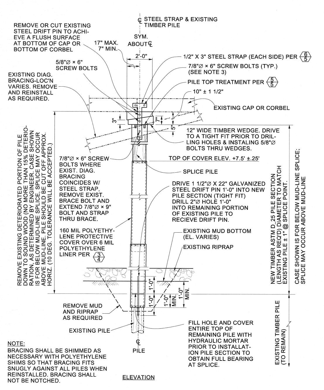
SPLICE PILE ("POST PILE" REPAIR METHOD)
